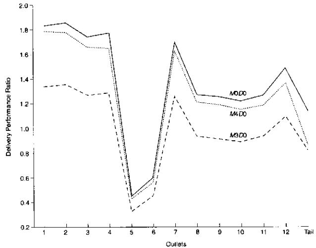
Figure 3.25: Simulated seasonal water deliveries to the tertiary units of the Masood Distributary as a result of management interventions at the main canal level. The results of Scenarios  $M3D0$  and  $M4D0$ , defined in Table 3.26, are compared with the reference scenario  $M0D0$ , by means of the delivery performance ratio (DPR).
