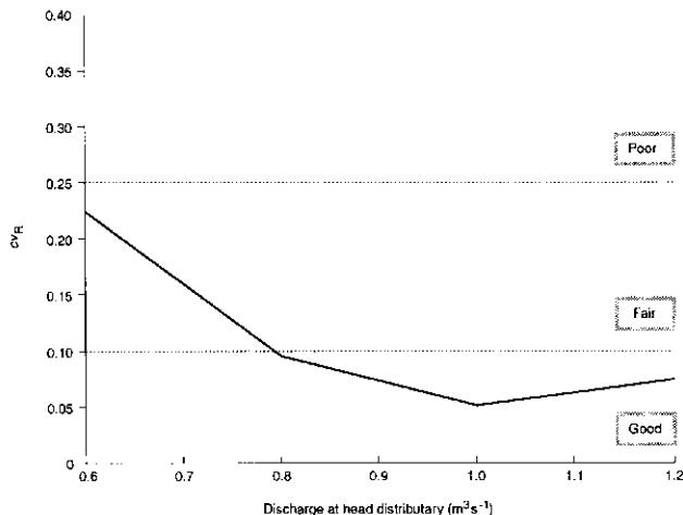
Figure 3.19: Evaluation of the simulated impact of the inflow at the head of a distributary in design conditions on the equitability of water distribution through the coefficient of variation,  $cv_R$  (after Visser, 1996). The performance criteria for  $cv_R$  are indicated.
