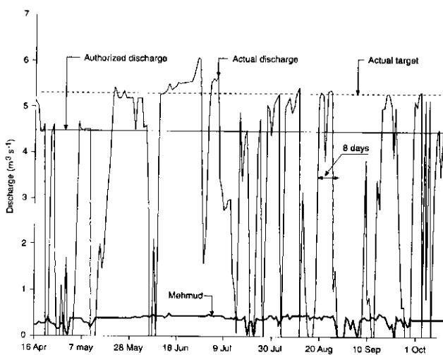
Figure 3.10: Comparison of actual discharge of the Fordwah Distributary of Kharif 1994 with the authorized discharge and the actual target discharge. The length of an 8-day supply period is indicated.
