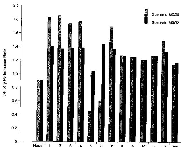
Figure 3.23: Comparison of simulated water deliveries for the actual situation (*MOD0*) and after intervention (*MOD2*) to outlets of the Masood distributary for Kharif 1994. The water deliveries are expressed as a delivery performance ratio (*DPR*).
