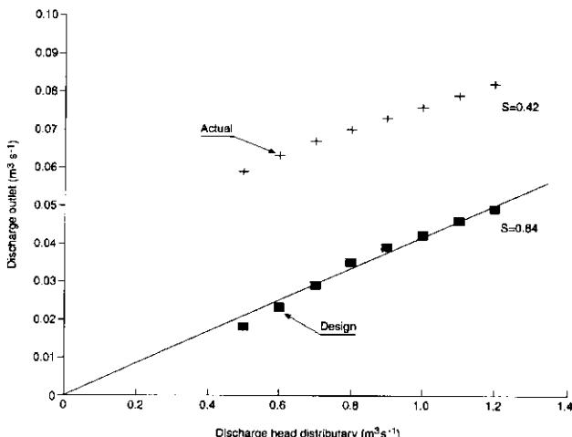
Figure 3.18: Sensitivity,  $S$ , of a tertiary offtake (fixed orifice) as a function of the discharge at the head of the distributary. The values for the design as well as the actual situation, for offtake 3700R of the Masood Distributary, have been calculated using the hydro-dynamic model SIC (after Visser, 1996).
