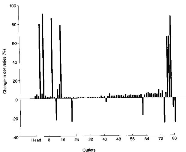
Figure 3.24: Comparison of simulated water deliveries of Scenarios *M0D0* and *M0D3* for the Fordwah Distributary for Kharif 1994, showing the effect of redimensioning selected outlets on the water distribution. The intervention serves to better target water supplies for salinity management.
