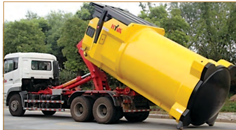
Container being lifted by the hook loader for disposal
