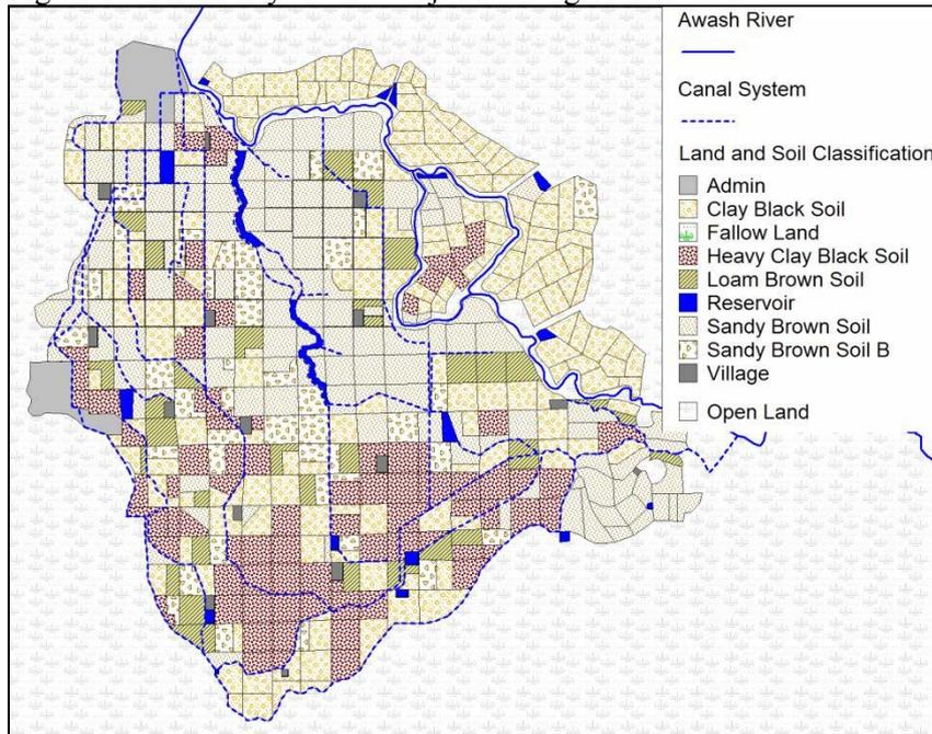
Figure 2: Scheme layout of Finchaa Valley Sugar Estate
