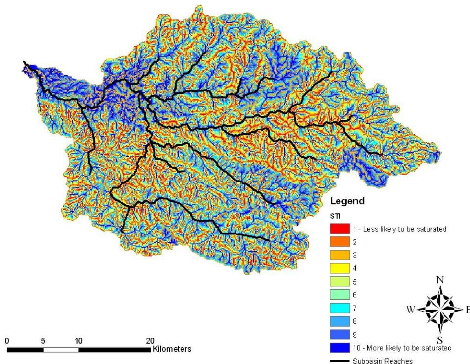
Figure 2: Soil topographic index for the Gumera basin
