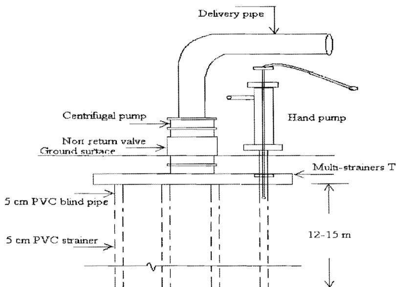
**Figure 3. A hand pump to diagnose the suction problems in the multi-strainers pumps.**
