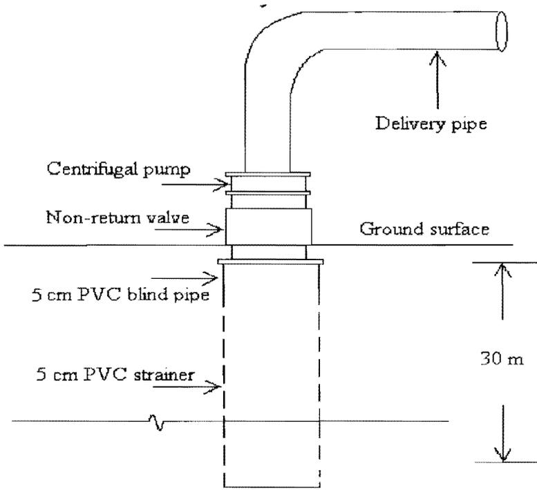
**Figure 1. Schematic diagram of a single strainer centrifugal pump.**
