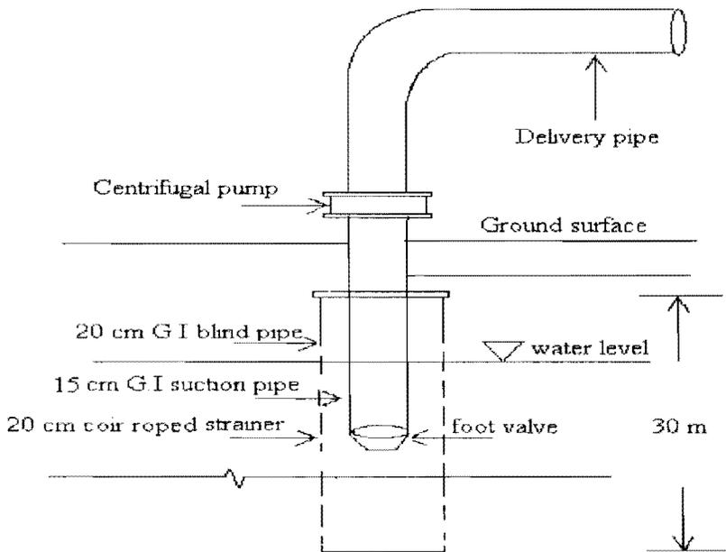
**Figure 4.** A schematic diagram of a tubewell with a suction assembly that is rarely used now.
