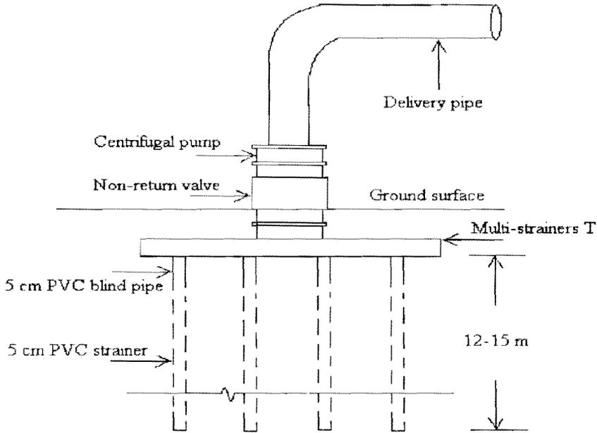
Figure 2. Schematic diagram of multi-strainers skimming well.
