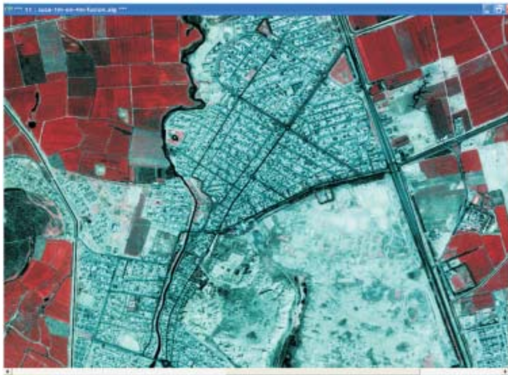
Figure 11. IKONOS 4-m data for watershed level studies. The image is in Karkheh River basin, Iran, covering the ancient historical city of Susa. Color key: RGB (FCC): 4,3,2. Data fusion technique involving the fusion of IKONOS multispectral 4-m and panchromatic 1-m.
