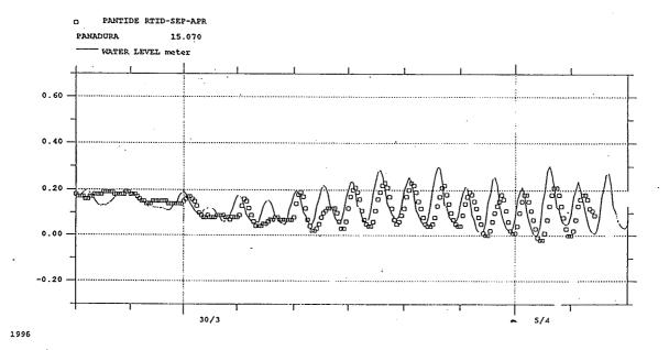
Figure 2: Panadura River: Example of Water Level Calibration
