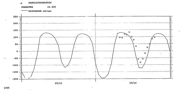
Figure 1: Panadura River: Example of Discharge Calibration
