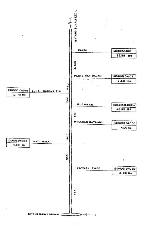
Figure 5. Matrix presentation of irrigation system information along a particular river
