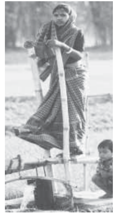
The treadle pump, a manually operated water pump, allows poor farmers to access groundwater to irrigate small plots of land. IWMI's research shows that this simple technology has the potential to put US$ 1 billion of new revenue directly into the hands of some of the poorest people in the world.
